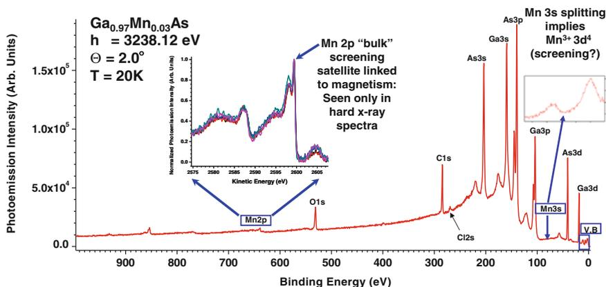
**Fig. 1.8** Survey spectrum from the dilute magnetic semiconductor  $\text{Ga}_{0.97}\text{Mn}_{0.03}\text{As}(001)$  with 3.2 keV excitation, and with *enlarged insets* from scanning longer on Mn 2p and 3s. Mn 2p reveals a sharp final-state screening peak only seen with hard X-ray excitation. Mn 3s show a doublet due to multiplet splitting that can be used to estimate the spin of Mn. Data from SPring-8 (From [40])
