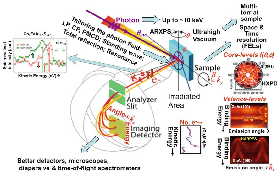
**Fig. 1.2** Schematic illustration of the different measurement modalities in photoemission, with *inset* examples discussed later in this and other chapters of this book. The core schematic from which this figure is derived is from Y. Takata
