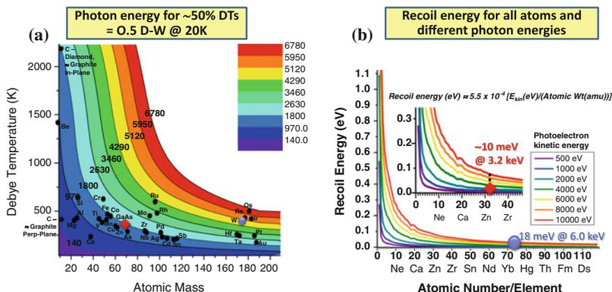
**Fig. 1.9** Calculated parameters for estimating the feasibility of ARPES at higher energies, including (a) contours for various photon energies to yield a photoemission Debye-Waller factor  $W(T)$  of 0.5 at 20 K, and (b) the recoil energy for all atoms as a function of photon energy. Values for two first demonstration cases W and GaAs studied with hard X-rays [39] are highlighted (From [55])
